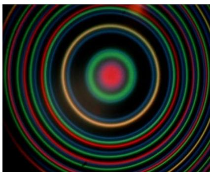
Figure 4. Fabry-Perot pattern with no filters or magnetic field.
