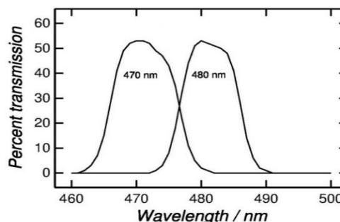
Figure 3. Transmission curves for the interference filters used. Data from Thorlabs, <http://www.thorlabs.com/>.
