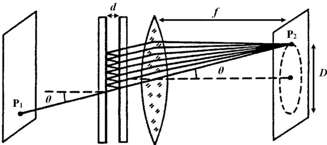
**Figure A1-3.** Light path through a Fabry-Perot-interferometer.
