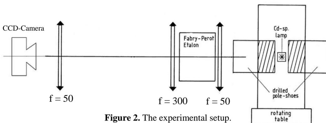
Figure 2. The experimental setup.
