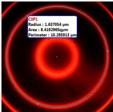
**Figure 5.** Fitting of the Fabry-Perot rings with the 3-point-circle tool in *Motic Images Plus*.
