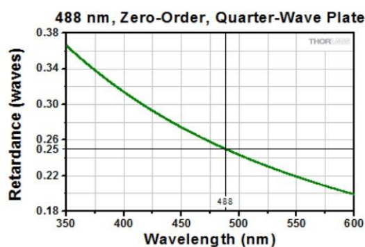
Figure 3b. Actual retardance for the plate that is \lambda/4 at 488 nm. Data from Thorlabs 4 .
