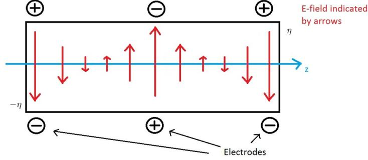
FIG. 53: Experimental sketch with 6 electrodes, the strength of the electric field are shown as red arrows.
