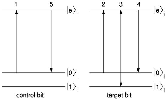
FIG. 2. A CNOT operation with qubit  $i$  as control and qubit  $j$  as target bit. The operation makes use of the following sequence of  $\pi$  pulses: (1)  $|0\rangle_i \leftrightarrow |e\rangle_i$ , (2)  $|0\rangle_j \leftrightarrow |e\rangle_j$ , (3)  $|1\rangle_j \leftrightarrow |e\rangle_j$ , (4)  $|0\rangle_j \leftrightarrow |e\rangle_j$ , and (5)  $|0\rangle_i \leftrightarrow |e\rangle_i$ . See text for explanation.
