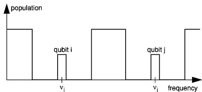
FIG. 1. A schematic diagram of a part of the inhomogeneously broadened spectrum of excitation frequencies to the excited state  $|e\rangle$  in rare-earth-metal ions in an inorganic crystal. Two qubits  $i$  and  $j$  are defined by two different transition frequencies in the spectrally hole-burnt structure.
