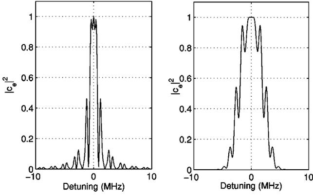
FIG. 3. Excitation by a composite pulse sequence  $90_{90}180_{180}90_{90}$  of rectangular pulses (left) and a composite pulse sequence  $92.50_{96.98}192.00_{6.86}92.42_{96.23}$  of Gaussian pulses (right). The total duration of both sequences is  $1.5 \mu\text{s}$ .
