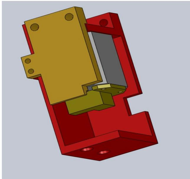
Figure 13: The pieces that are removed during sample swap.
