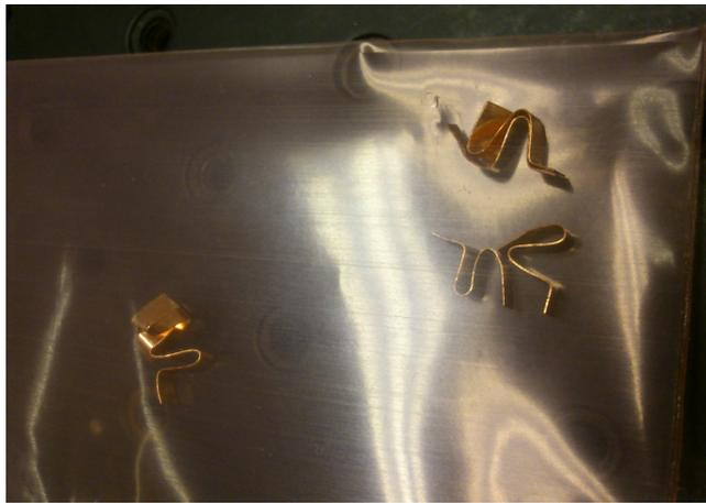
Figure 29: Oxygen annealed copper links that will connect the sample holder and thermal link
