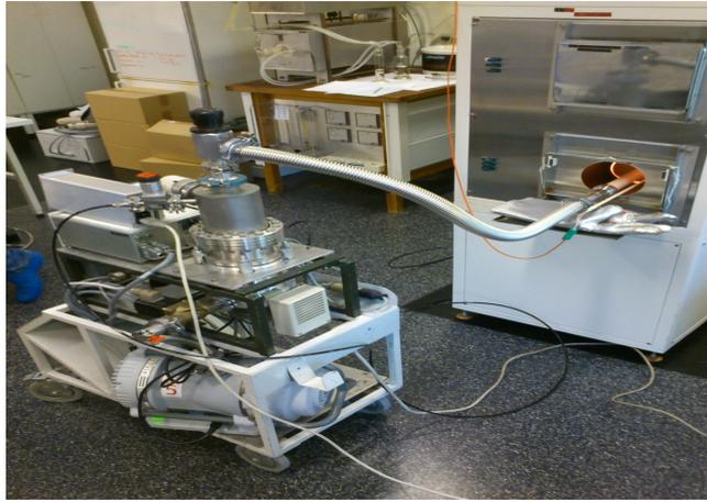
Figure 18: Oxygen annealing system.
