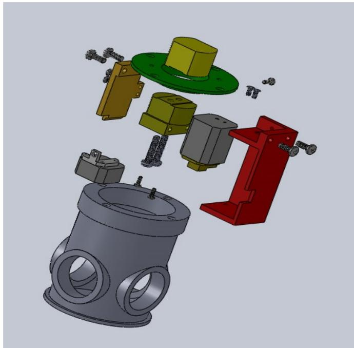
Figure 28: Exploded complete model of the system inside the cryostat
