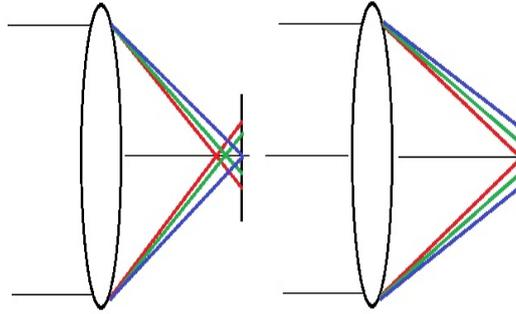
Figure 4: Greatly exaggerated picture showing the effects of chromatic aberration.
