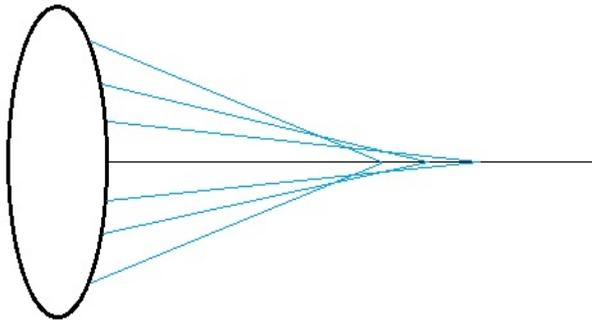
Figure 6: Spherical aberration
