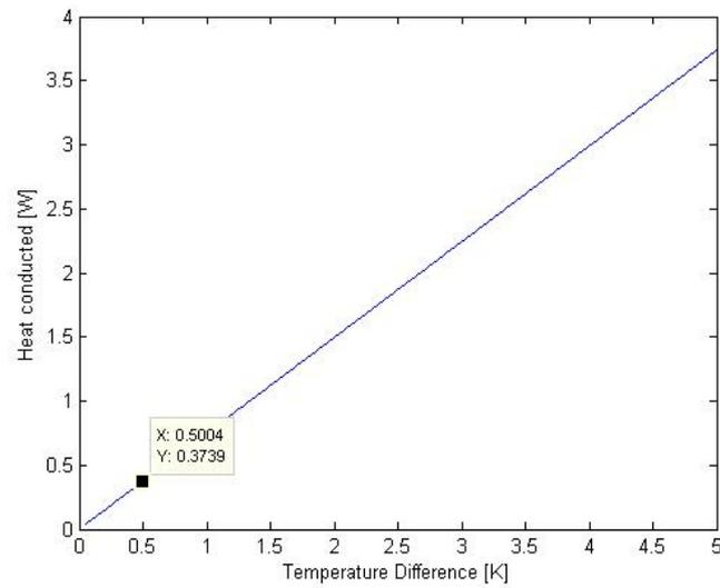
Figure 17: Heat conductivity for the thermal link with high purity copper.
