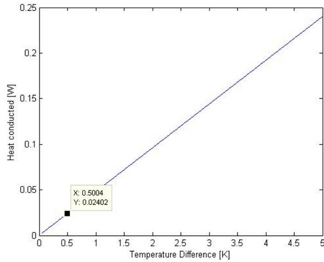
Figure 16: Heat conductivity for the thermal link with high purity copper.
