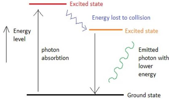
Figure 1: Energy transitions for fluorescence.
