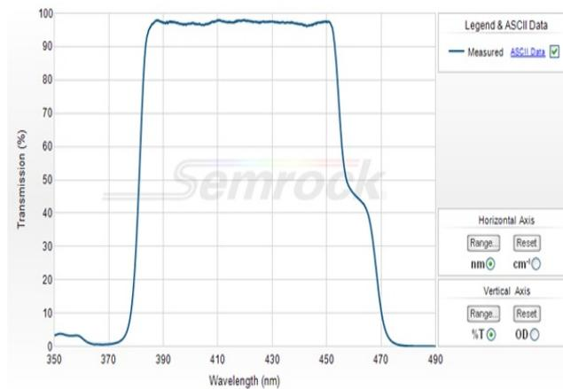
Figure 26: Transmission graph for the dichroic beam splitter brightline from Semrock. Figure from [18]
