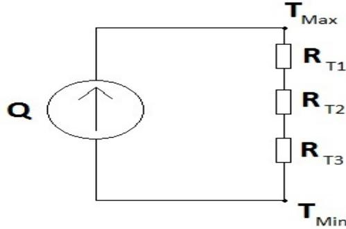
Figure 7: Equivalent schematic for thermal resistance conversion calculation in the form of a circuit diagram.
