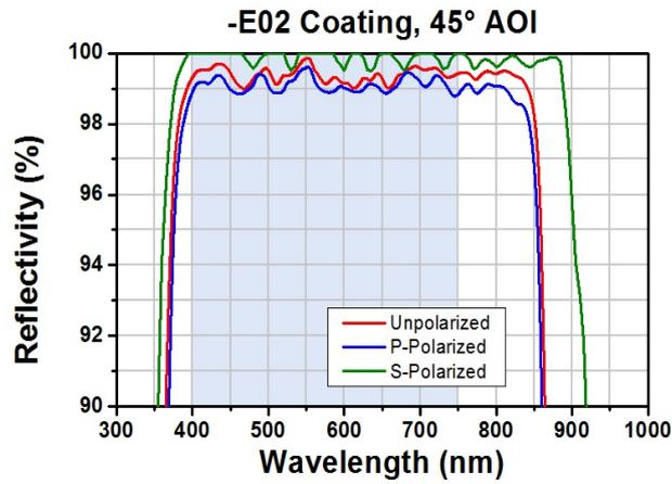
Figure 25: Transmission graph for the dichroic mirrors E02. Figure from [17]
