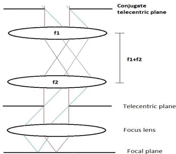
Figure 3: Illustration of how a telecentric system behaves. Observe that the colors of the beams have nothing to do with wavelength of the light.
