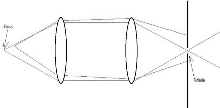
Figure 2: Picture showing how a pinhole blocks out light out of focus.
