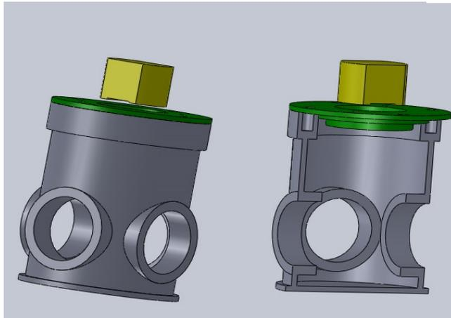
Figure 10: Model of the cryostat.
