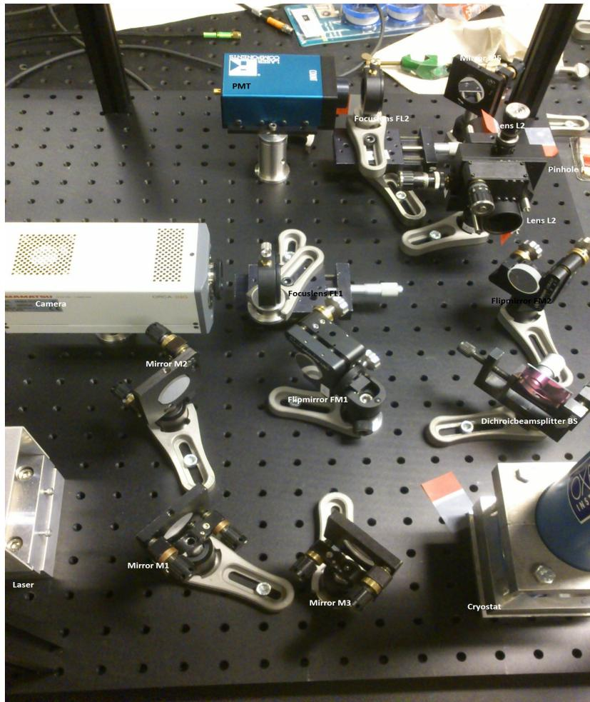
Figure 24: The complete optical setup
