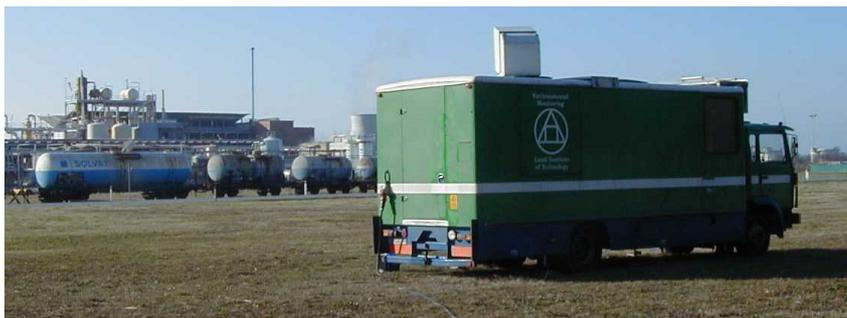
Fig. 1. The mobile lidar system in a field campaign in Rosignano Solvay, Italy.
