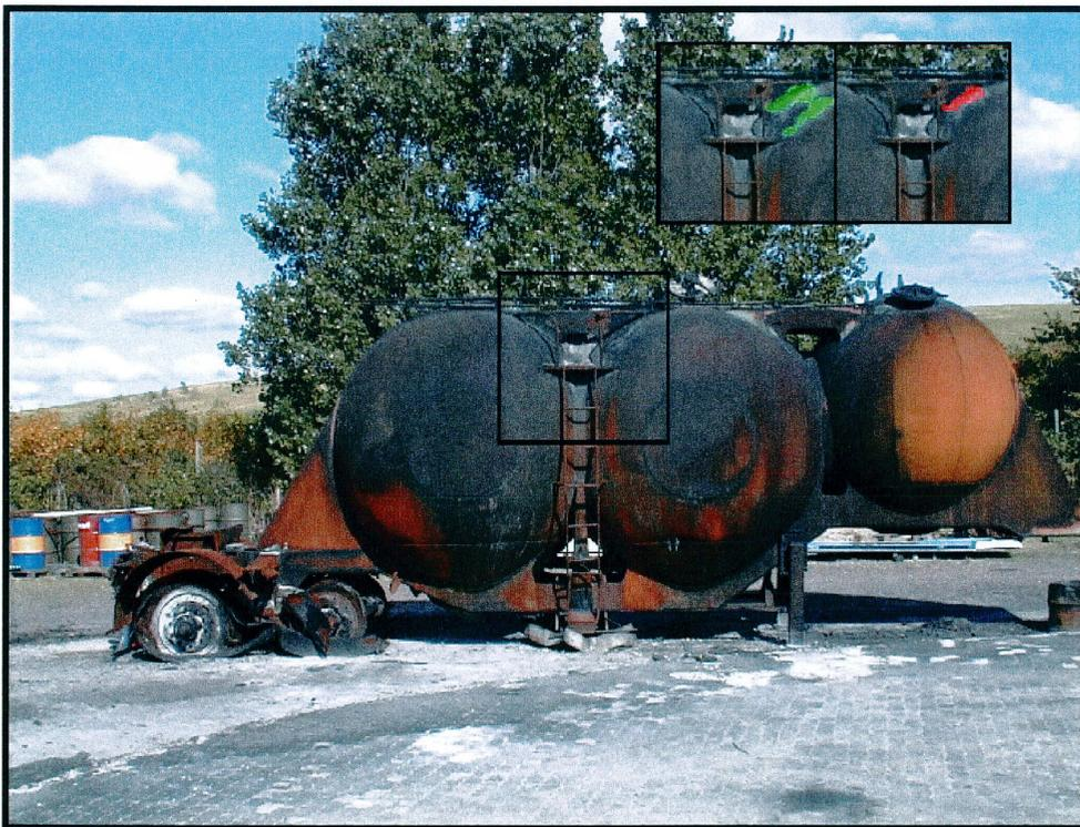
Fig. 37. A burnt out gas tanker with spectrally interfering ammonia and ethene gas leaks. The ammonia gas is gas-correlated and seen in the upper right image.
