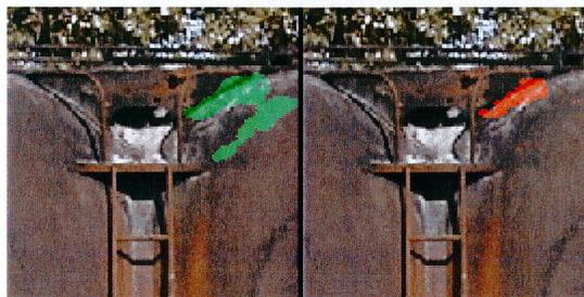
Fig. 11. (1.9 MB) Simultaneous imaging of ammonia and ethylene leaks showing the isolation of the ammonia flow using the gas-correlation technique. Measurement conditions: Time 17:25, Air temperature 19.2 °C, Surface temperature 31.5 °C, Relative humidity 50 %, Ammonia gas flow 15 l/min, Ethylene gas flow 10 l/min, ZnSe gas cell with ammonia 1 atm., Filter: Spectrogon LP9200.
