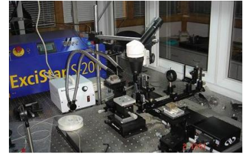
Figure 5.3. The FBG fabrication system at Zhejiang University.
