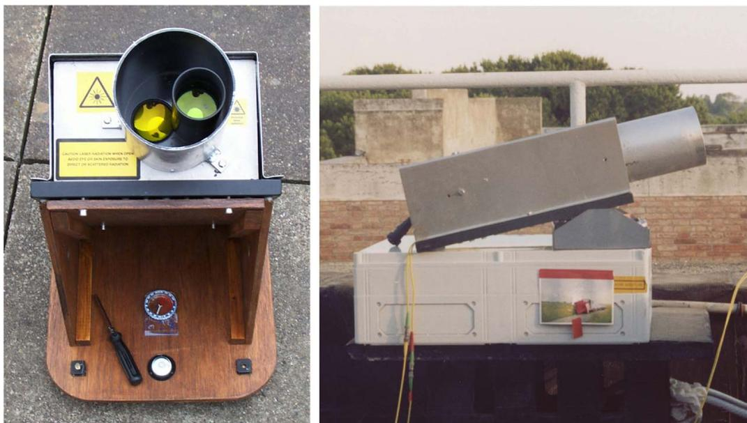
Fig. 1. Optical head of Doppler Lidar system. The beam is normally directed at  $60^\circ$  to the horizon. In the image to the right, an angle of elevation of  $11.9^\circ$  has been improvised.
