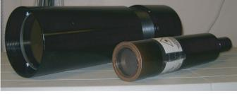
**Figure 4.4.** A photograph of the two beam expanders; the smaller one used for DIAL and LIF and the larger one used for LIBS measurements.
