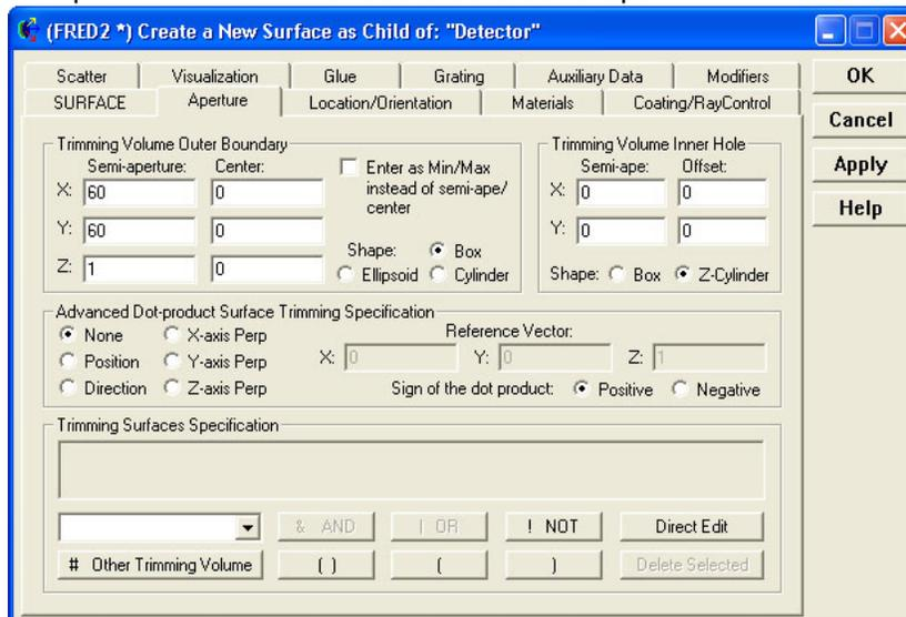
Move the detector plane +300 mm in the Z direction by selecting the Location/Orientation page tab and append a location/direction primitive modifier (right click inside the location tab and select append).
