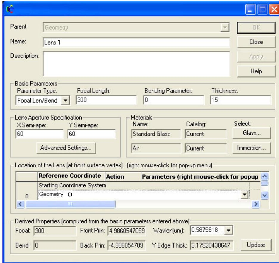
Change the focal length to 300 mm, the thickness to 15 mm and the X and Y Semi-apertures to 60 mm. The analyzed image will now look something like below, but I've increased the number of rays.
