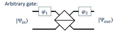
Combining the two elements can create any superposition state
