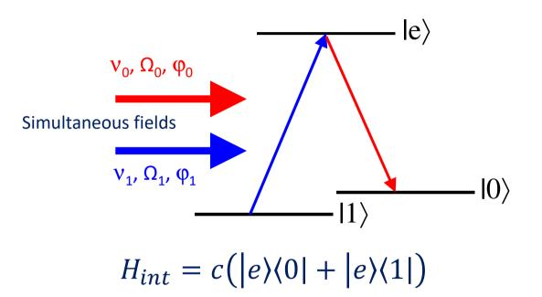
Superpositions:Interactions: $|B\rangle = |0\rangle + |1\rangle$  $\langle e|H_{int}|B\rangle = 2c$  $|D\rangle = |0\rangle - |1\rangle$  $\langle e|H_{int}|D\rangle = 0$
