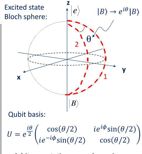
= Arbitrary rotation around an axis on the equator
