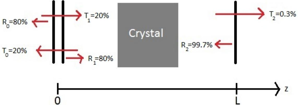
FIG. 20: Crystal inside a cavity, reflectivity and transmission shown in percent.
