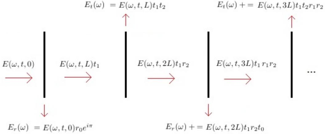
FIG. 21: Model for the cavity.
